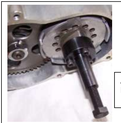
Remove button head screws. Take Lever Assembly off.
