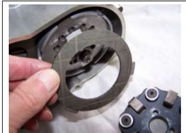
Inspect friction disc and replace when worn below .088" Note: it is not necessary to remove drive hub when replacing friction disc.
