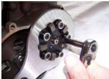
Remove button head screws. Take Lever Assembly off.
